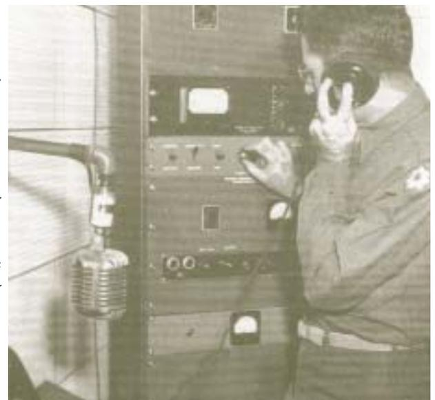
First Lt. Raymond H. "Woody" Hull calibrating the rack-mounted equipment used for two-room audiometry during the early days of the Borden program.
