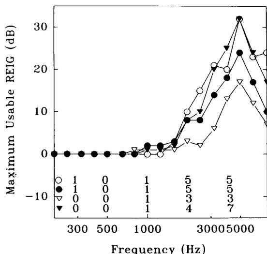
**Figure 7** Maximum usable REIG permitted by four nonoccluding earmolds (Westone #12: open circle, Westone #13: closed circle, Tube: open inverted triangle, and Oticon E43: closed inverted triangle) coupled to the Oticon E43 hearing aid. The magnitudes of the standard deviation are shown.
