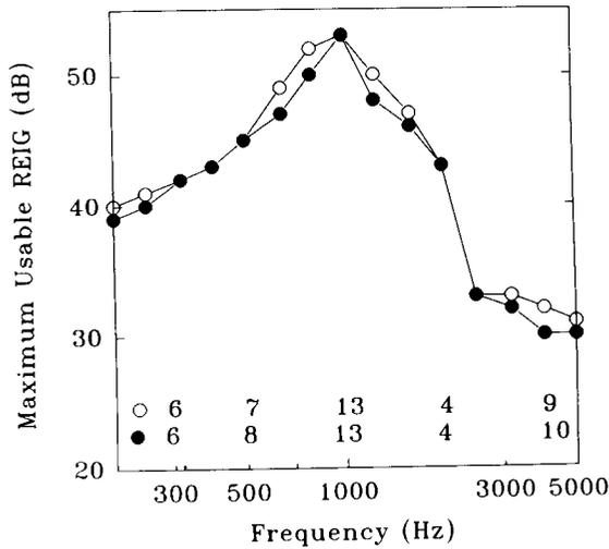
**Figure 4** Maximum usable REIG permitted by the skeleton earmold with (open circle) and without (closed circle) the helix lock. The magnitudes of the standard deviation are shown at the bottom of the figure.
