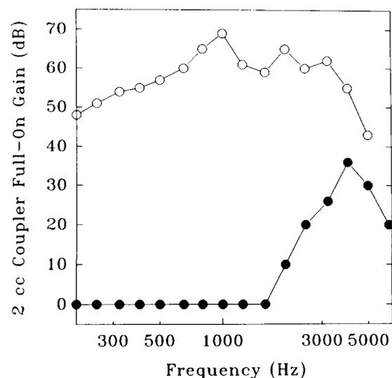
**Figure 1** Two-cc coupler full-on gain curves for the Phonak Super-Front PPCL (open circle) and Oticon E43 (closed circle) hearing aids used in the study.
