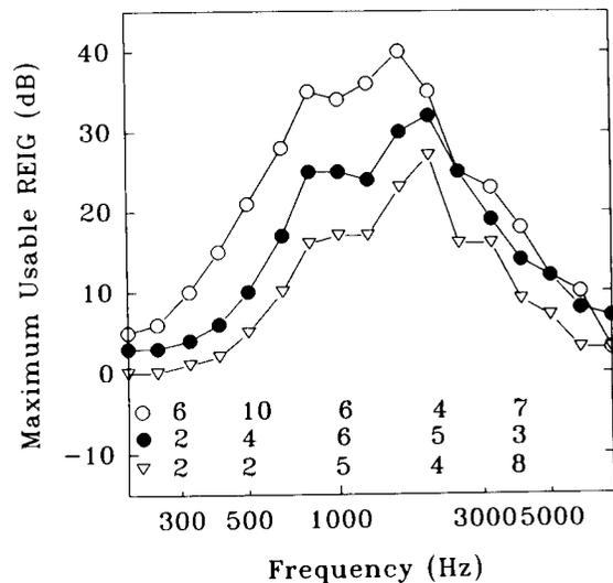
**Figure 6** Maximum usable REIG permitted by three nonoccluding earmolds (Westone #12: open circle, Westone #13: closed circle, and Tube earmold: open inverted triangle) coupled to a Phonak Super-Front PPCL hearing aid. The magnitudes of the standard deviation are shown.
