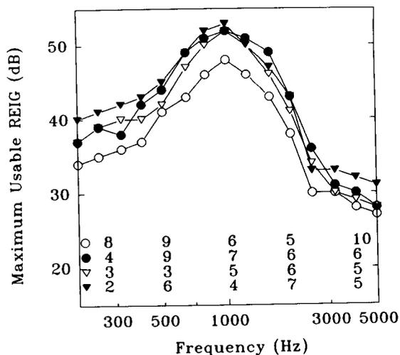
**Figure 2** Maximum usable REIG permitted by the standard (open circle), shell (closed circle), canal (inverted open triangle), and skeleton (closed inverted triangle) earmolds (no vent). The magnitudes of the standard deviation ( $\sigma_{n-1}$ ) for each earmold at 250, 500, 1000, 2000, and 4000 Hz are shown at the bottom of the figure.
