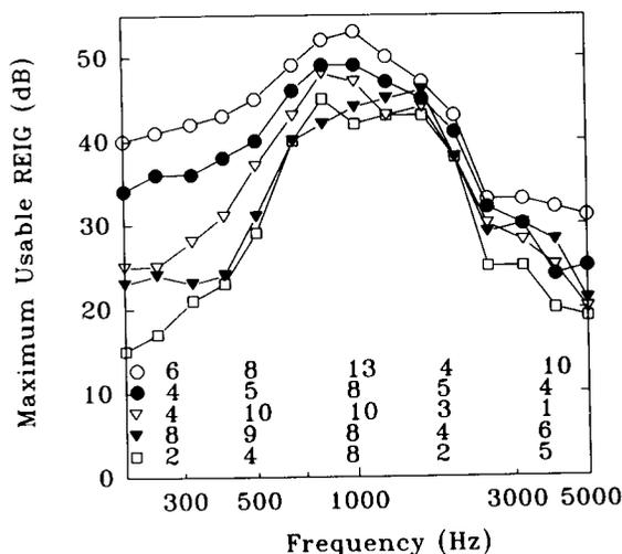
**Figure 3** Maximum usable REIG permitted by the skeleton earmold with closed SAV (open circle), pressure vent (closed circle), 1-mm (open inverted triangle), 2-mm (closed inverted triangle), and 3-mm (open square) vents. The magnitudes of the standard deviation are shown at the bottom of the figure.
