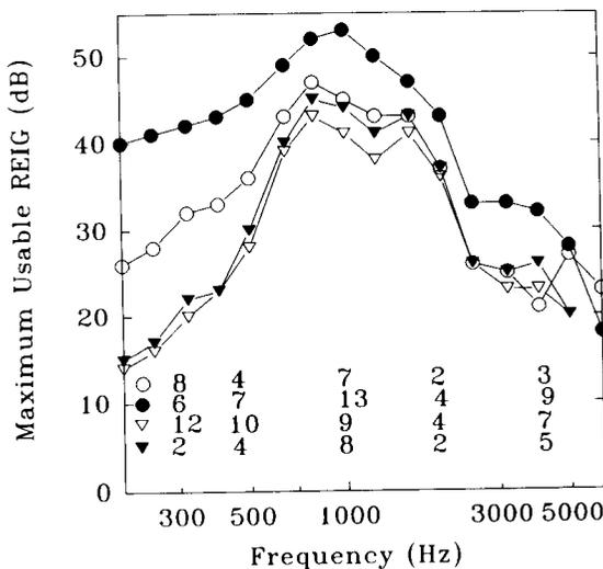
**Figure 5** Maximum usable REIG permitted by the skeleton earmold modified in four manners: with crus and SAV closed (closed circle), with crus and 3-mm vent (closed inverted triangle), without crus and SAV closed (open circle), and without crus and 3-mm vent (open inverted triangle). The magnitudes of the standard deviation are shown.
