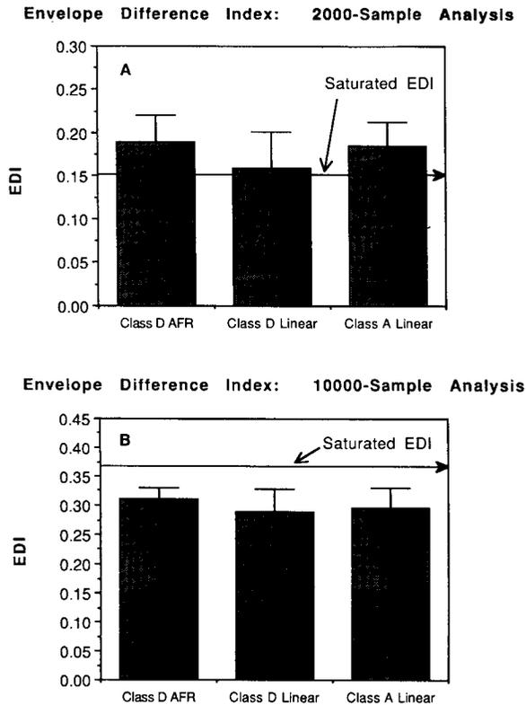
**Figure 4** Mean envelope difference index values obtained across hearing aids. Panels A and B represent 2000-sample (beginning with stimulus onset) and 10,000-sample analysis intervals, respectively. The horizontal line within each panel represents the EDI associated with a saturated linear hearing aid. Error bars represent one standard deviation.
