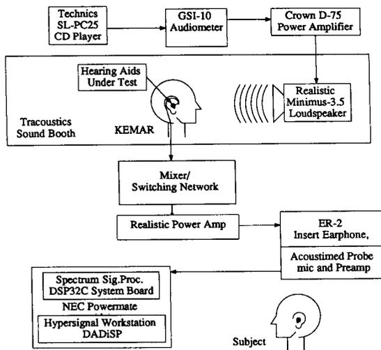
**Figure 1** Block diagram of the experimental apparatus used to present test stimuli and to record and analyze real-ear data.
