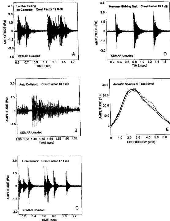
**Figure 2** Examples of temporal waveforms of test stimuli, recorded unaided on KEMAR. A, Lumber falling on concrete. B, Automobile collision at the moment of impact. C, Seven firecracker bursts. D, Three strikes of a hammer to a nail. E, Acoustic spectra of test stimuli.
