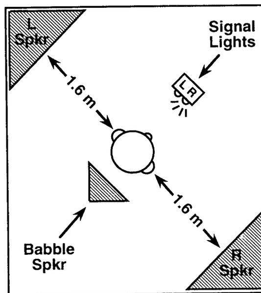
**Figure 2** Arrangement of apparatus for the cued-listening task.
