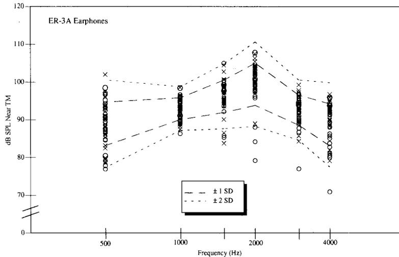
**Figure 2** Individual SPL measured near the eardrum at 500 to 4000 Hz for the ER-3A earphone ( $N = 50$ ). The "O" represents the right ear and "X" represents the left ear. Also included are  $\pm 1$  and 2 standard deviations (SD).
