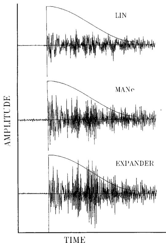
**Figure 5** Amplitude-time waveforms of the postvocalic /t/ burst after processing by the LIN, MANe, and Expander (EXP) circuits. Each waveform is overlaid by a half-Hamming window that marks the onset of the burst and highlights amplitude differences. The rms level of each vowel was digitally equated at 70 dB SPL; therefore, burst amplitude differences were the result of processing by the different hearing aid circuits.
