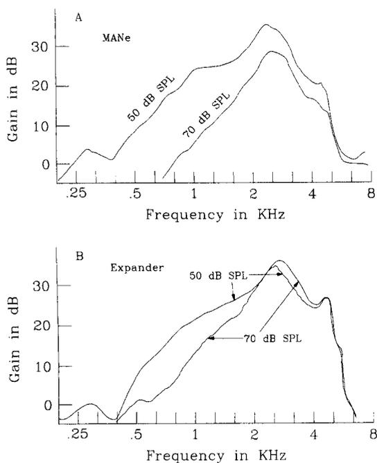
**Figure 2** Frequency response curves on the 2-cc coupler for the Manhattan II with experimental modifications (MANe; Part A) and for the EXP hearing aid (Expander; Part B) with broadband stimulus input levels of 50 dB SPL and 70 dB SPL.
