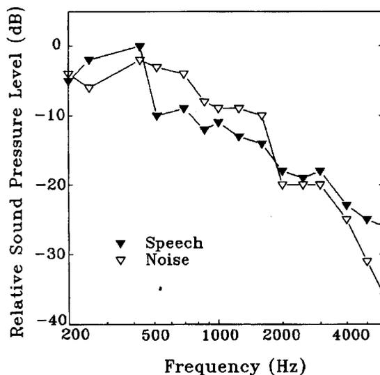
**Figure 2** Spectra of the speech (▼) and noise (▽) stimulus used in the study (measured in 1/3-octave band).
