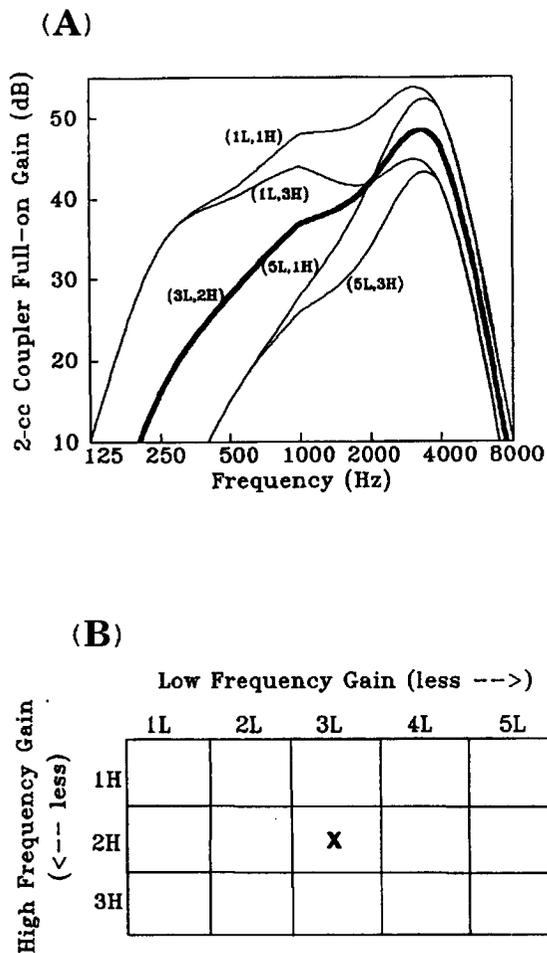
**Figure 1** Two-cc coupler full-on gain curves (A) and matrix (B) showing the range of low- and high-frequency gain changes on the experimental hearing aid.
