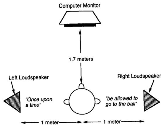
Figure 1 Arrangement of testing apparatus.
