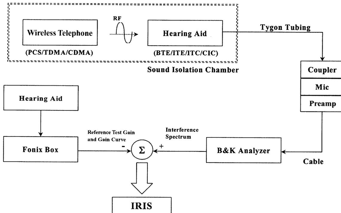
**Figure 3** Determination of the input referenced interference spectrum.
