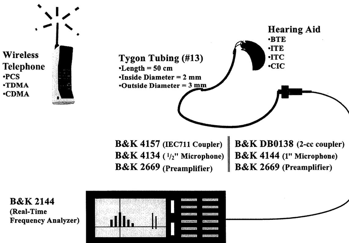
Figure 2 Equipment for acoustic measurements of hearing aid interference.
