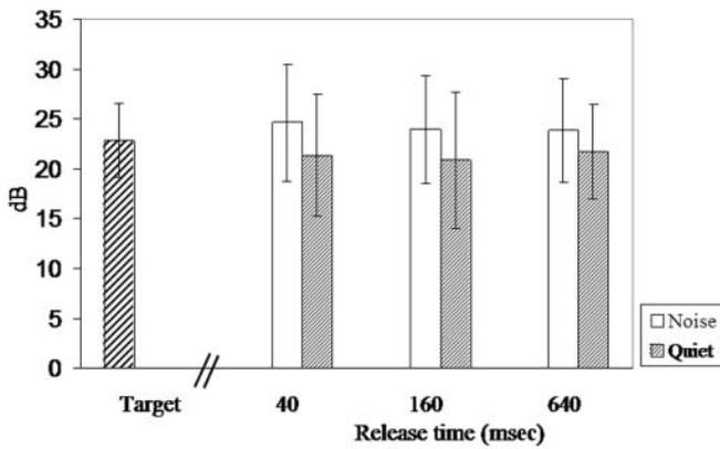
**Figure 3.** Average real ear gain at 58 frequencies from 750 to 4000 Hz. The striped bar represents mean target gain and the white and shaded bars mean gain selected by the subjects for each release time condition for noise and quiet, respectively. Error bars are +/- 1 SD.
