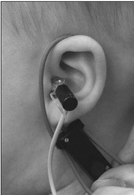
**Figure 3.** Real-ear measurement portion of the real-ear-to-coupler difference (RECD). The eartip/probe-tube unit is inserted into the ear canal, and a signal is delivered from the RE770 transducer. The difference between the SPL measured in the coupler and the SPL measured in the real ear are the RECD values across frequency.
