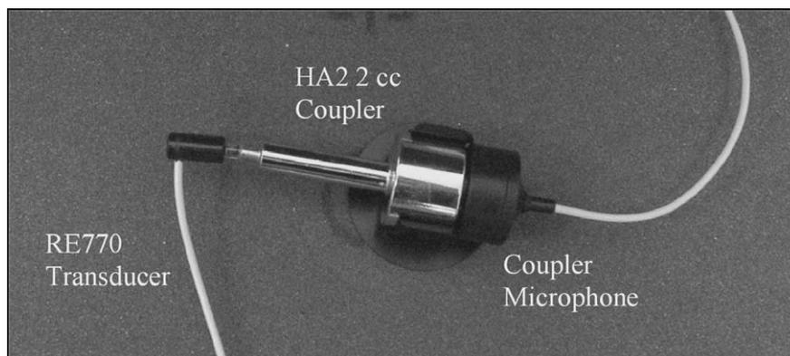
**Figure 1.** Coupler measurement portion of the real-ear-to-coupler difference. The RE770 transducer is connected to the HA-2 2-cc coupler that is connected to the coupler microphone of the Verifit. A signal is delivered to the coupler to measure the coupler response across frequency.
