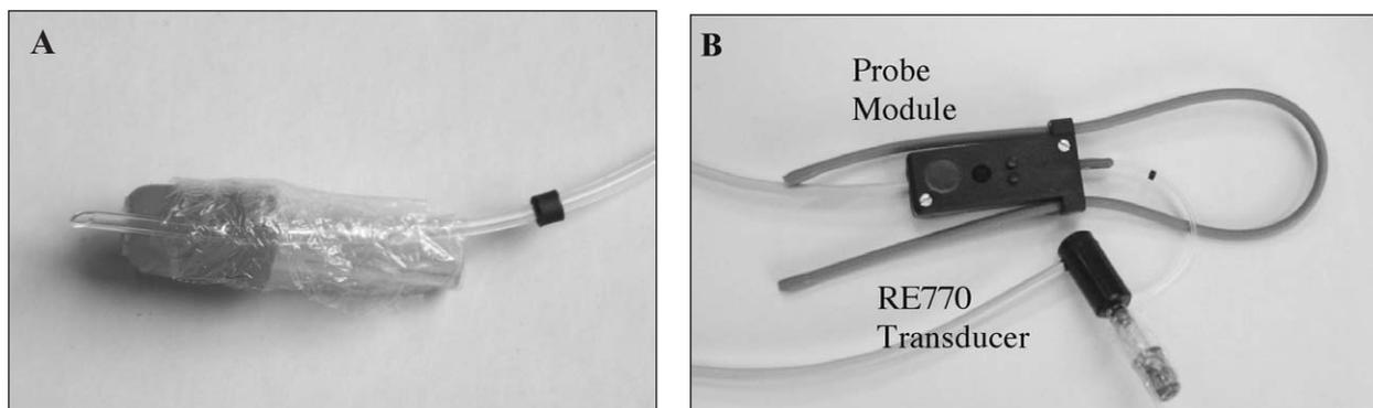
**Figure 2.** (A) Probe-tube coupled to a 3.5 mm ER-10 otoacoustic emission eartip using plastic film. (B) Eartip/probe-tube unit connected to the Verifit real-ear module and RE770 transducer for measurement of the real-ear portion of the real-ear-to-coupler difference (RECD).
