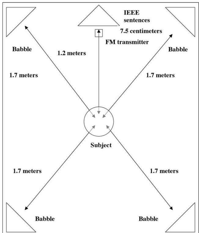
**Figure 1.** A diagram of the loudspeaker configuration used in this investigation.
