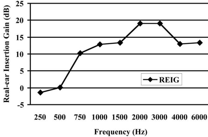
**Figure 2.** Real-ear insertion gain (REIG) obtained for one subject at a volume control setting of 6 using an 80 dB SPL input of composite noise.
