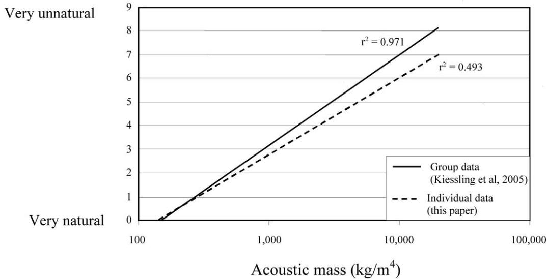
**Figure 7.** Linear regression analysis of perceived occlusion (y) versus individual acoustic mass data (x).
