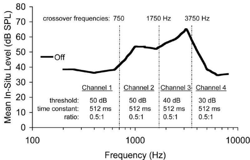
**Figure 2.** Expansion parameters determined by the Starkey software and crossover frequencies between the first and second, second and third, and third and fourth channels of each hearing instrument. Mean in-situ levels averaged across ears for 13 of the 15 participants for the expansion off condition are shown for reference purposes.
