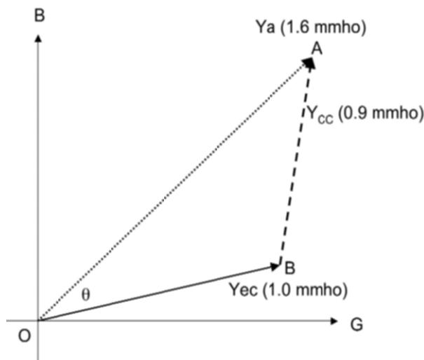
**Figure 1.** Graphical representation of admittance vectors OA and OB. OA minus OB equals BA, which represents the component compensated static admittance ( $Y_{CC}$ ).
