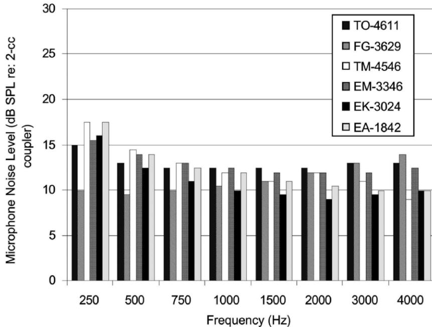
Figure 5. Approximate microphone noise levels of various Knowles microphones as taken from their datasheets.
