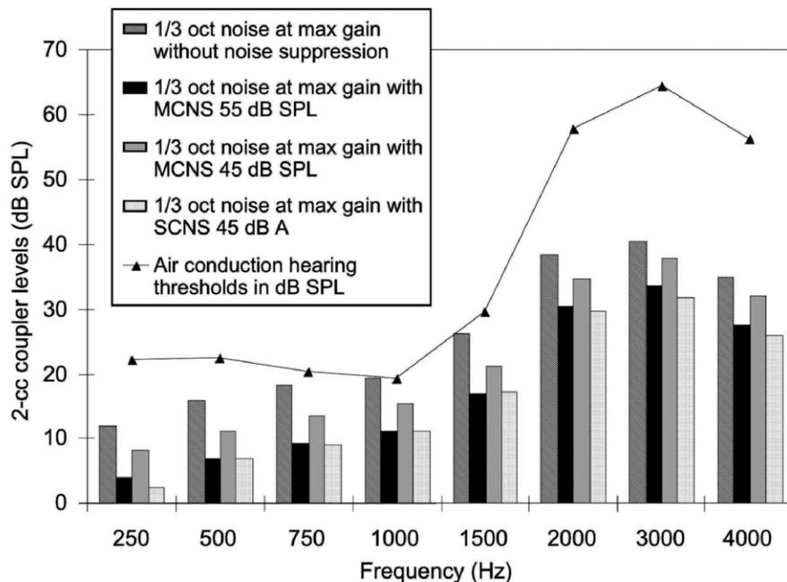
**Figure 4.** Microphone noise levels at the output of the aid with expansion OFF, SCNS, MCNS 45, and MCNS 55, and right ear air conduction thresholds (triangles) for participant 5.
