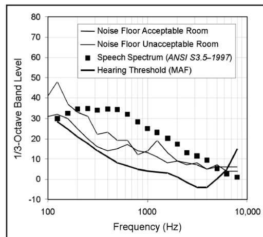
**Figure 3.** Comparison of noise floors in subjectively acceptable and unacceptable rooms. Noise floor overall level in the acceptable room was 35 dBA. In the unacceptable room the noise floor overall level was 26 dBA. Minimum audible field (MAF) curves have been superimposed for reference purposes.
