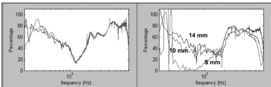
**Figure 8.** Effect of test–retest measures and probe insertion depth. Left panel: Power reflectance with three consecutive tests after probe removal and reinsertion to the same depth each time. Right panel: Power reflectance with three consecutive tests after probe removal and reinsertion to 14, 10, and 5 mm depths, respectively.
