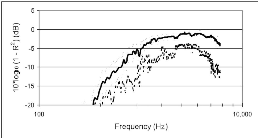
**Figure 3.** Average transmittance (chirp stimulus) for ears with normal ear status ( $n = 138$ ) shown with the solid line; 95 percent confidence intervals are shown with dotted lines. Comparison group is ears with poor status ( $n = 21$ ; dashed line).
