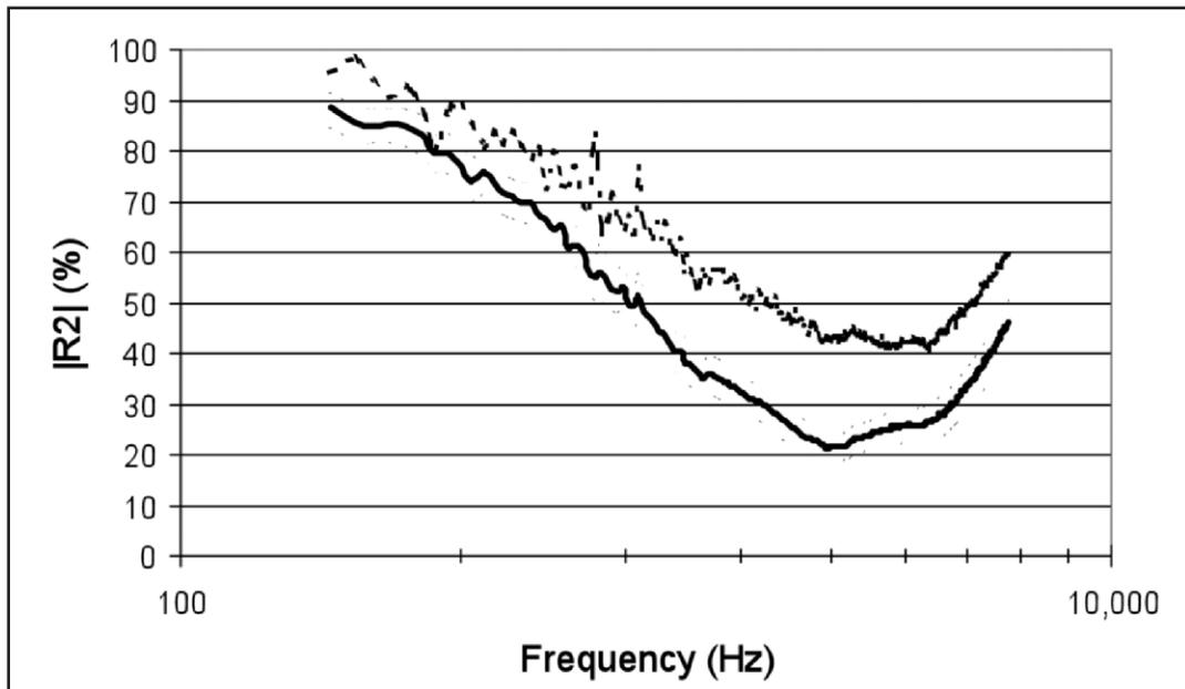
**Figure 1.** Average power reflectance (chirp stimulus) for ears with normal ear status (n = 138) shown with the solid line; 95 percent confidence intervals are shown with dotted lines. Comparison group is ears with poor status (n = 21; dashed line).
