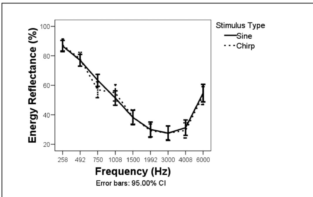
Figure 6. Average power reflectance for broadband chirp compared to sine wave stimuli for all ears with normal status in which both stimulus types were completed (n = 93). Error bars are 95 percent confidence intervals.
