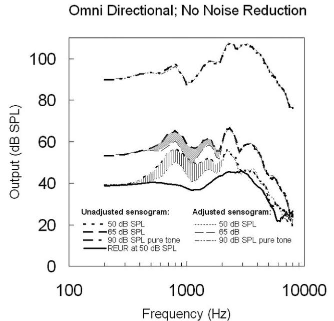
**Figure 1.** Real-ear output of the hearing aid to a 50 and 65 dB SPL speech-shaped composite noise input. The OSPL90 curves and the real-ear unaided response (REUR) at a 50 dB SPL input level are also shown.
