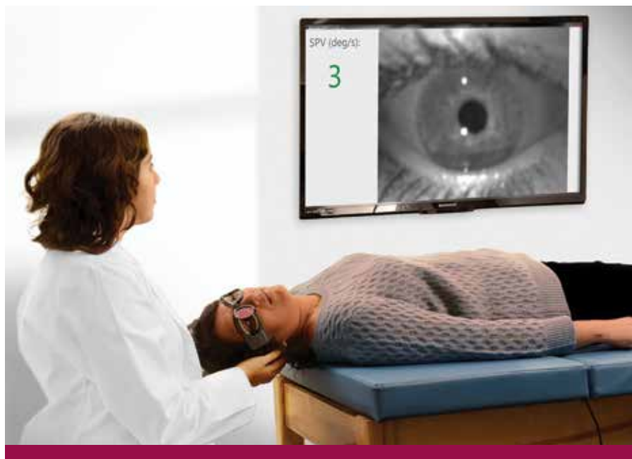
External monitor displaying the eye video and real-time slow phase velocity.
