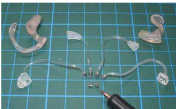
FIGURE 6. Concha-Line/Cymba-Line earmold with an integrated conic slotted metal sleeve and replacement instrument.
