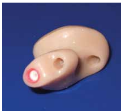
FIGURE 1A. CIC systems with two parallel short vents.
